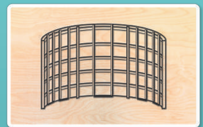
Radial framed formwork
