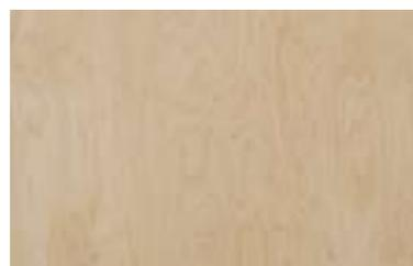
**Practically without defects:** some healthy inter-grown knots up to 25 mm in diameter, insignificant brown veins and dropped out knots up to 5 mm in diameter are admitted.
